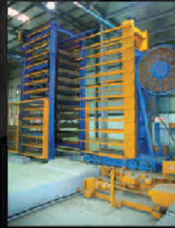
6- Elevator / Finger Car
